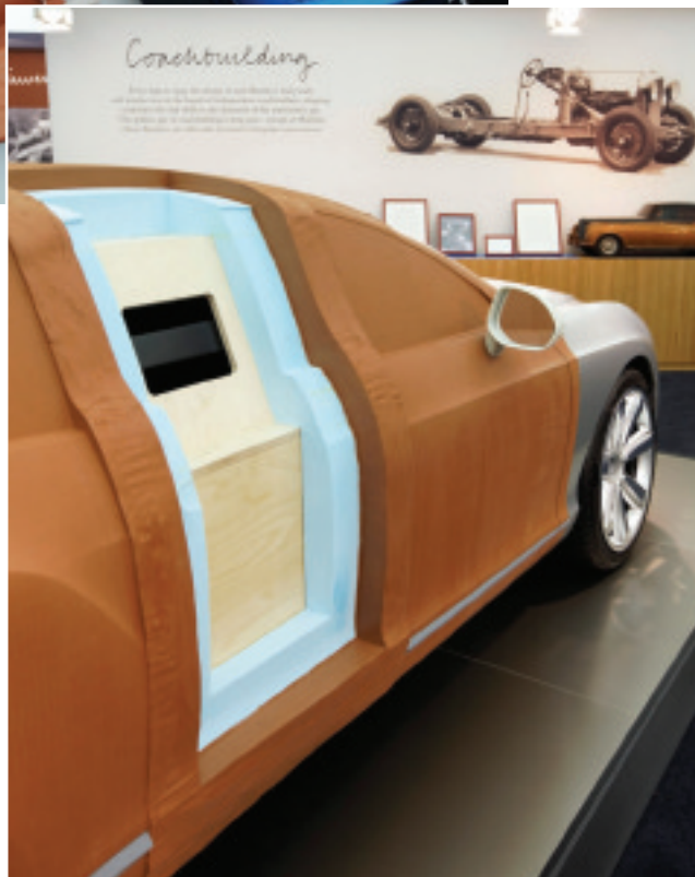
Bentley uses rapid prototyping early in the design process and in conjunction with full scale clay models
