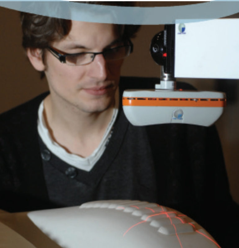
Laser scanning a surface (above) to produce a point cloud and then a surface model (below right) to enable simulations and then parametric models to be produced. These can then be edited and manipulated to improve upon the design (below)
